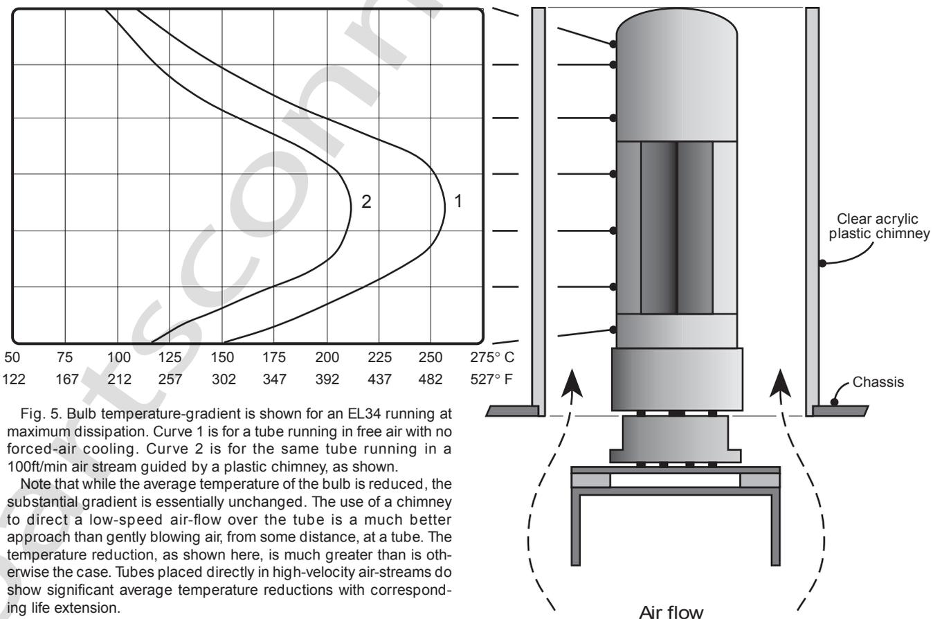
Fig. 5. Bulb temperature-gradient is shown for an EL34 running at maximum dissipation. Curve 1 is for a tube running in free air with no forced-air cooling. Curve 2 is for the same tube running in a 100ft/min air stream guided by a plastic chimney, as shown.
