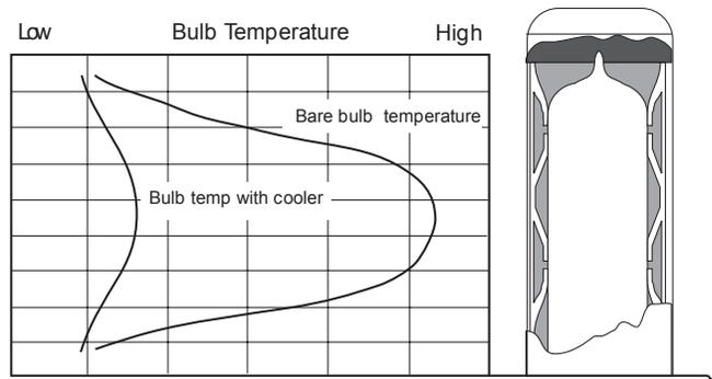
Fig. 4 . Tube-surface temperature gradient with proper cooling.
